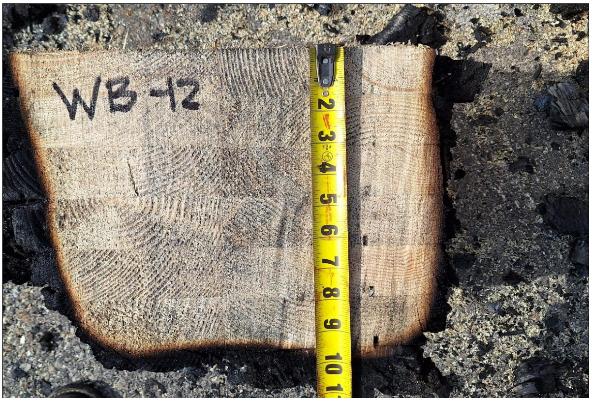
Figure B-12. View of Beam Cut 12 in. from End of Beam, Exposed 9.5 in. of Good Wood.
