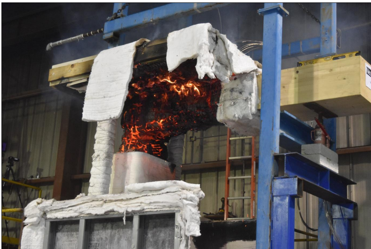
Figure B-7. View of Assembly during Removal from Furnace.
