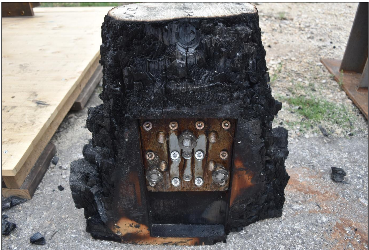
Figure B-10. Column with Male Self-Made Wiehag Connector , Posttest.
