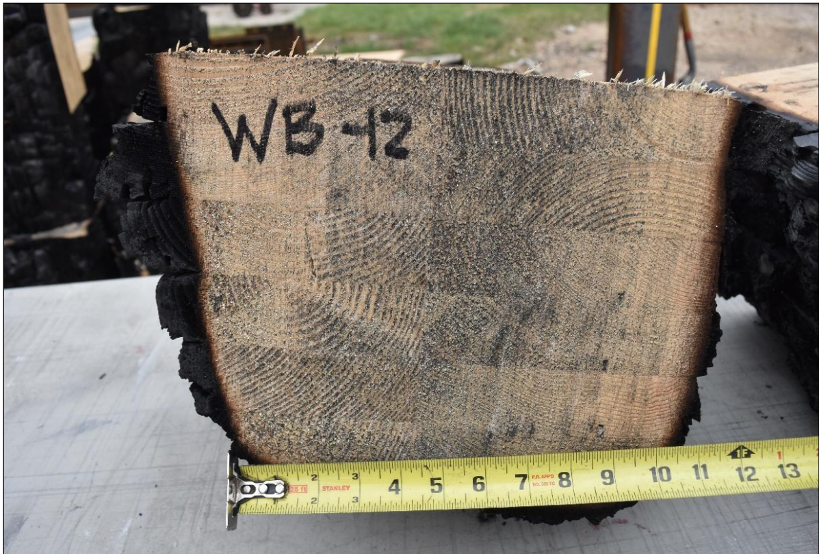
Figure B-11. View of Beam Cut 12 in. from End of Beam, Exposed 10.25 in. of Good Wood.
