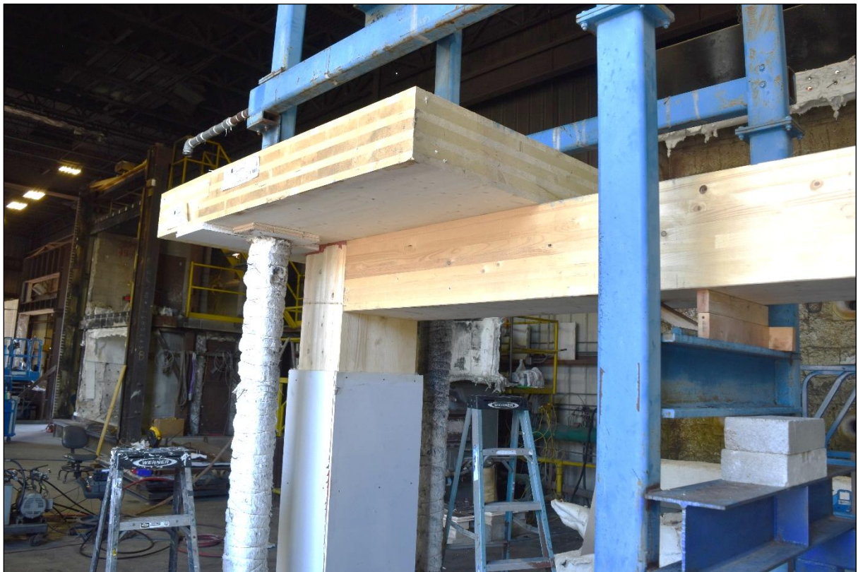
Figure B-3. Beam and Column, and CLT Panel Installed in Frame.
