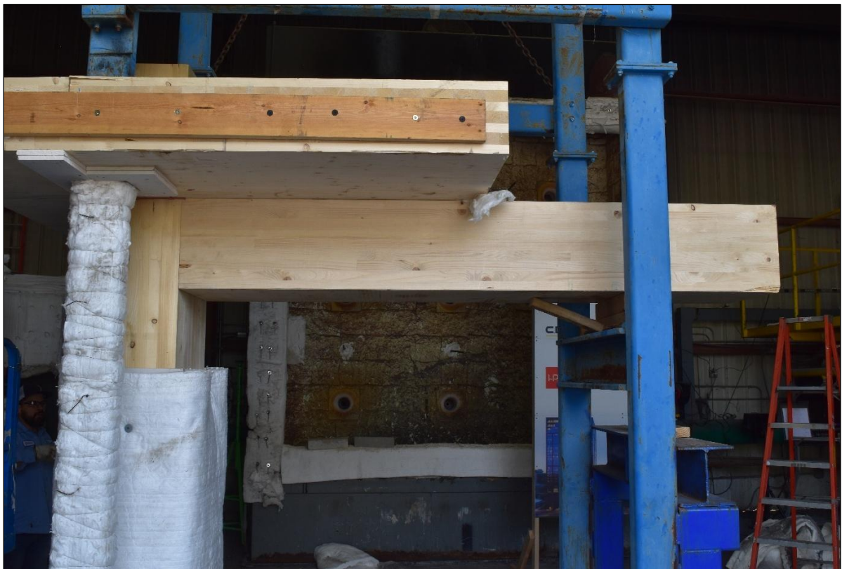
Figure B-2. Beam and Column, and CLT Panel Installed in Frame.
