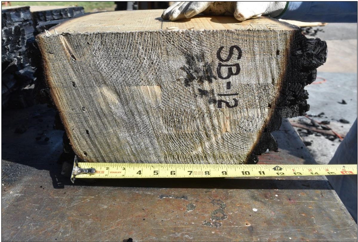
Figure B-11. View of Beam Cut 12 in. from End of Beam, Exposed 10 in. of Good Wood.
