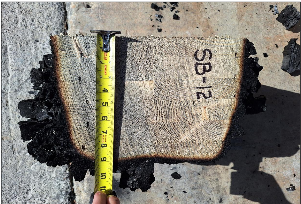
Figure B-12. View of Beam Cut 12 in. from End of Beam, Exposed 8.8 in. of Good Wood.
