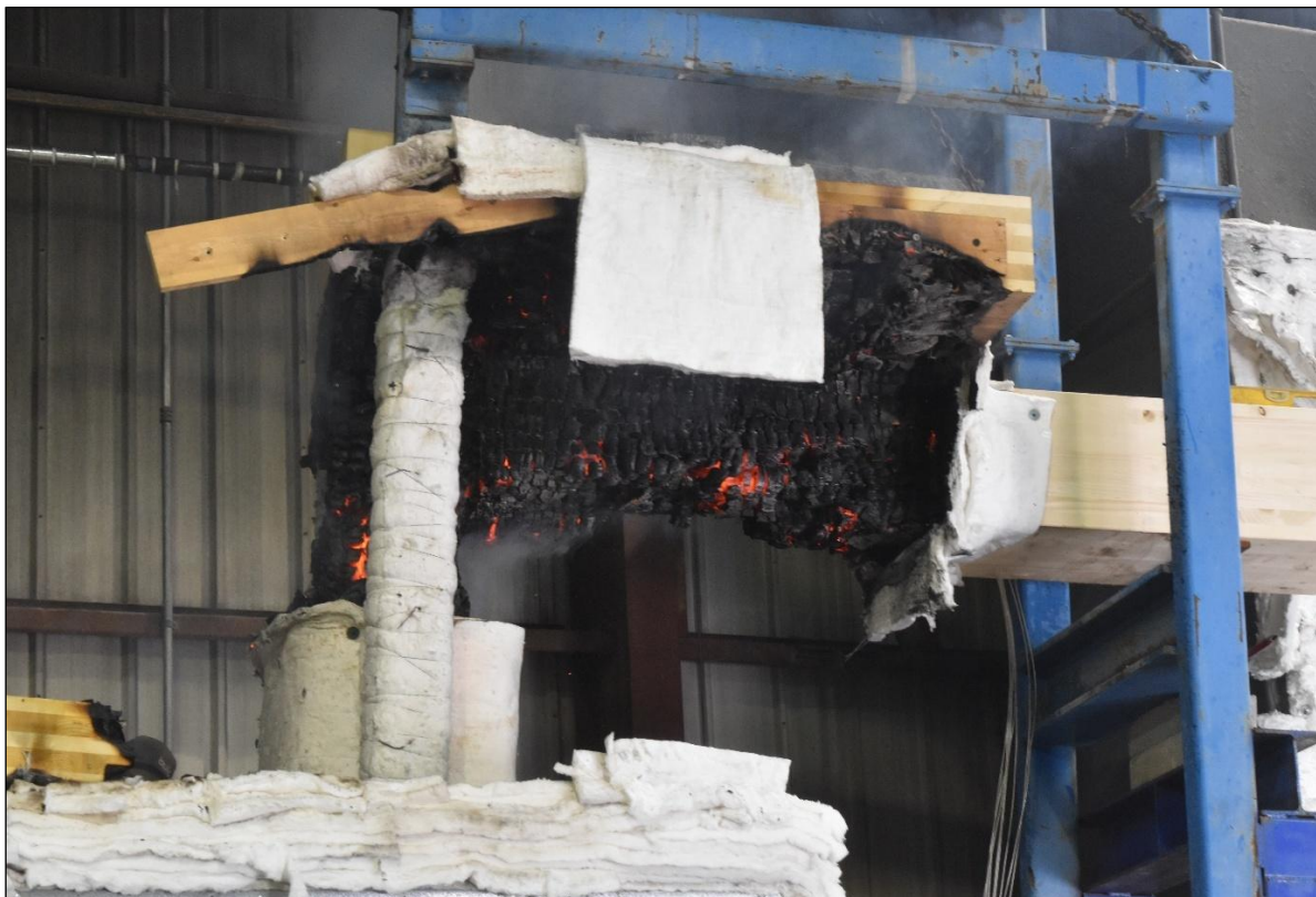
Figure B-7. View of Assembly during Removal from Furnace, following Removal of Rear Section of CLT.
