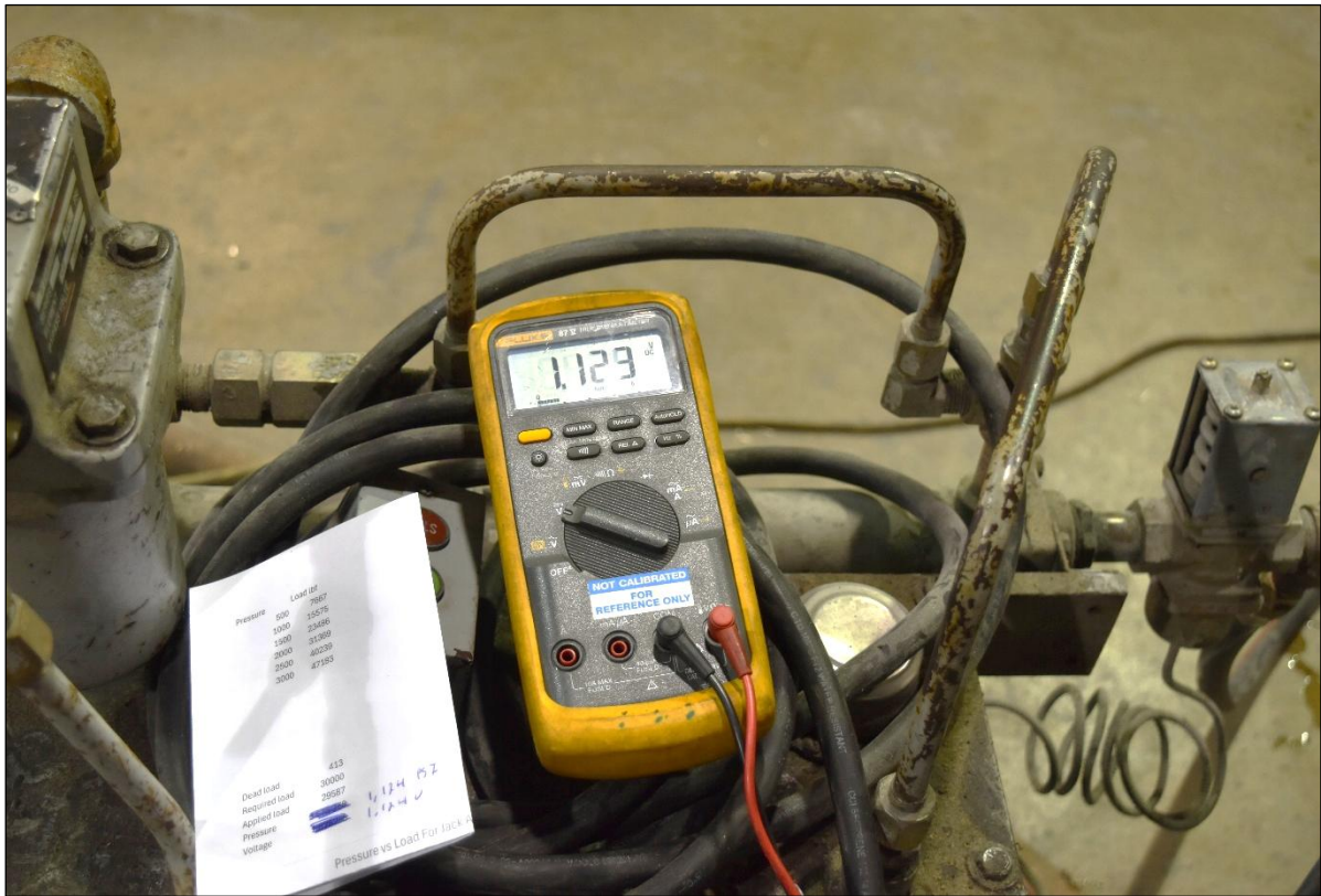
Figure B-5. View of Millivolt Output from Loadcell.
